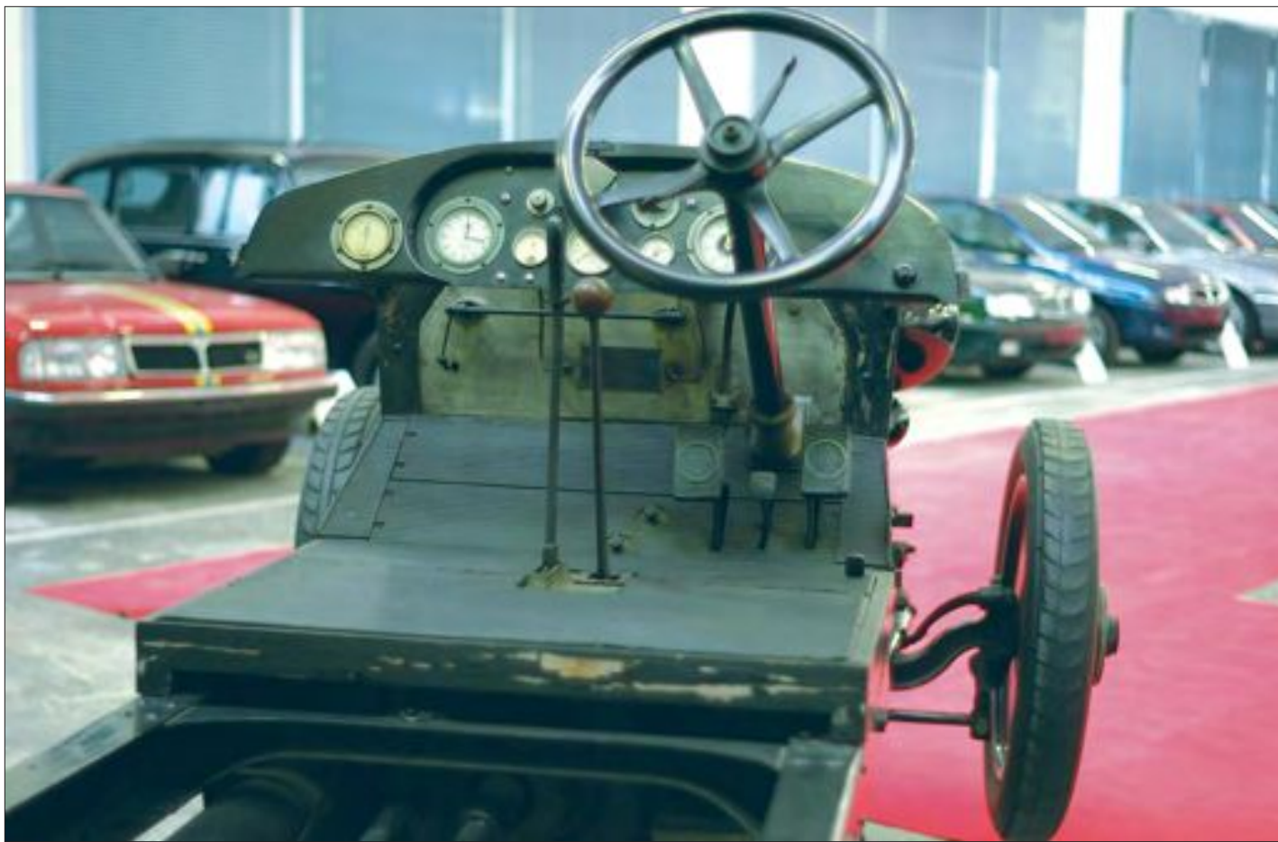
Above: Tri-Kappa chassis, with cast aluminum firewall for structural rigidity. The Tri-Kappa was the first Lancia with a V engine.
