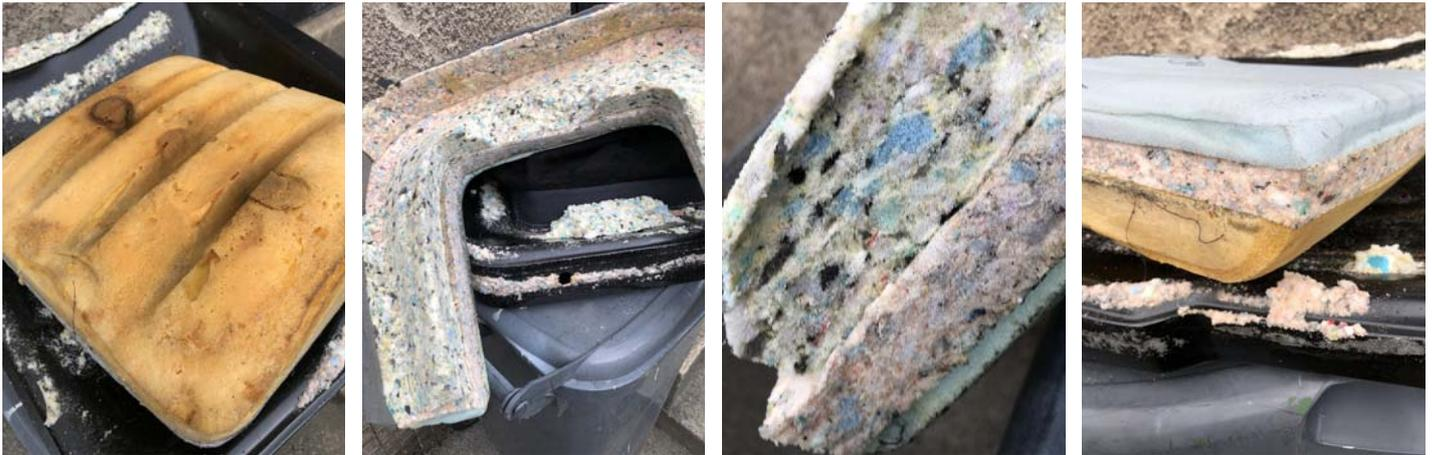
Rather than Norm's seats being glued to the metal base, my seat covers have a binding strip (mill board?) sewn to the reverse of the leather, so the binding is slipped/pulled over the pressed steel lip around the base of the seat and that keeps it taught. I started with the driver's seat and used the lessons of this one, when sorting out the passenger seat – trial and error!
